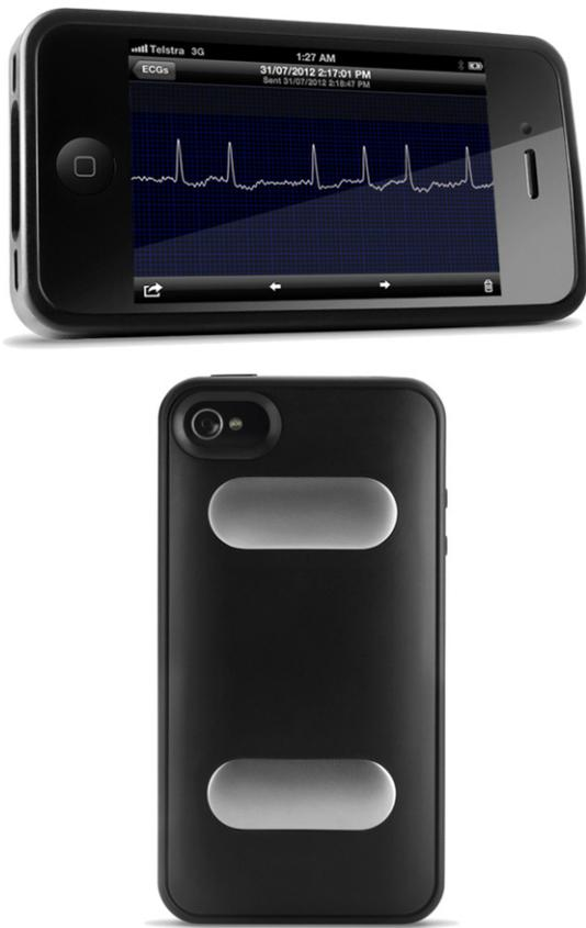
**Fig. 1.** iPhone single lead (Lead I) ECG showing AF. Electrodes are part of the AliveCor iPhone case on the reverse of the phone and correspond to the positive and negative poles of lead I.
